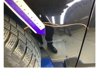
Çamurluk, sol, Çamurluk, sol > Ezik
