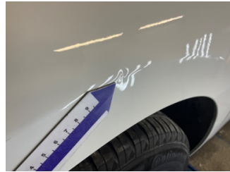
Çamurluk, sol, Çamurluk, sol > Ezik
