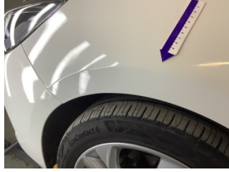
Çamurluk, sol, Çamurluk, sol > Ezik
